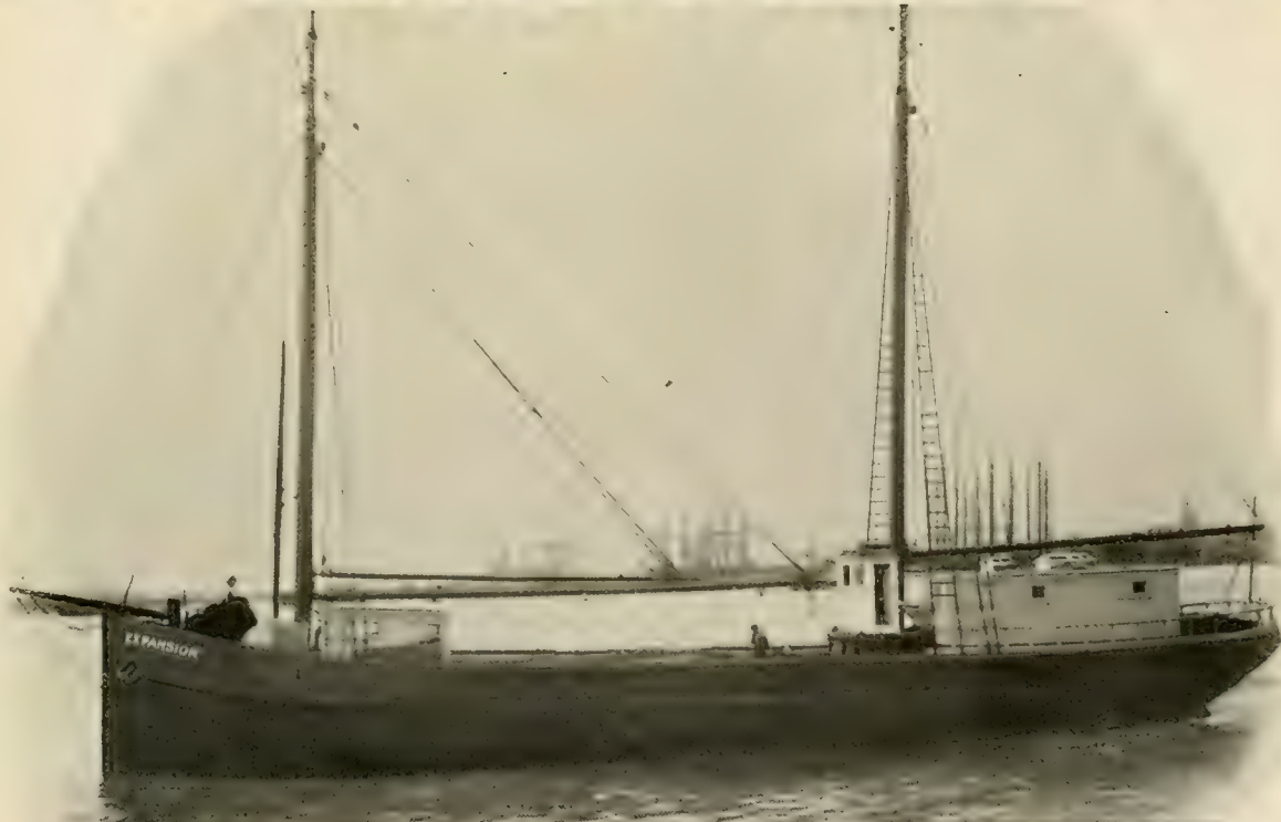
"Expansion," Largest Cannery Tender on the Pacific Coast. 112 ft. long, 24 ft. beam, 9 ft. depth of hold. Twin Screw Two 65 H. P. ATLAS Engines.
